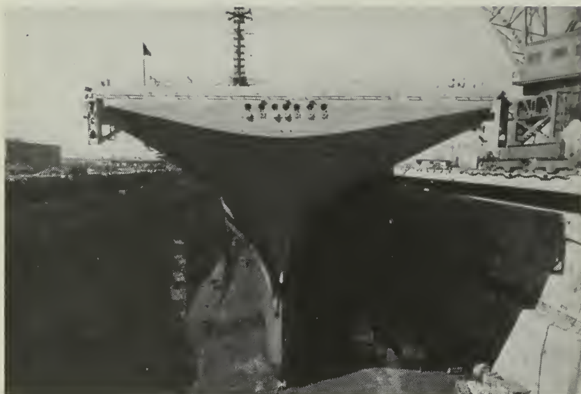
BOTTOMS OUT —USS Kearsarge (CVA 33) stands high and dry on keel blocks in U. S. Naval Shipyard, Long Beach, Calif., as she gets her hull cleaned.
